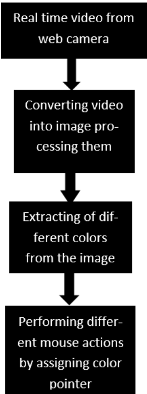
Figure 6.2. The Basic Block diagram of system
